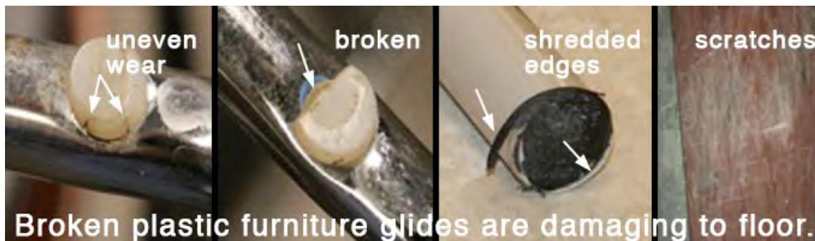
The rule for floor protector selection is simple: Hard floor protectors (plastic or metal) for soft-surface (carpeted) flooring and soft protectors (felt) for hard-surface floors.
