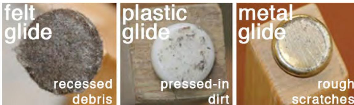
This opinion is based on my forty years of flooring industry experience, from sales and installation to manufacturer technical services and independent expert troubleshooter. In most cases of flooring failure problems, incorrect, damaged or uncared-for floor protectors contribute to the problem.
