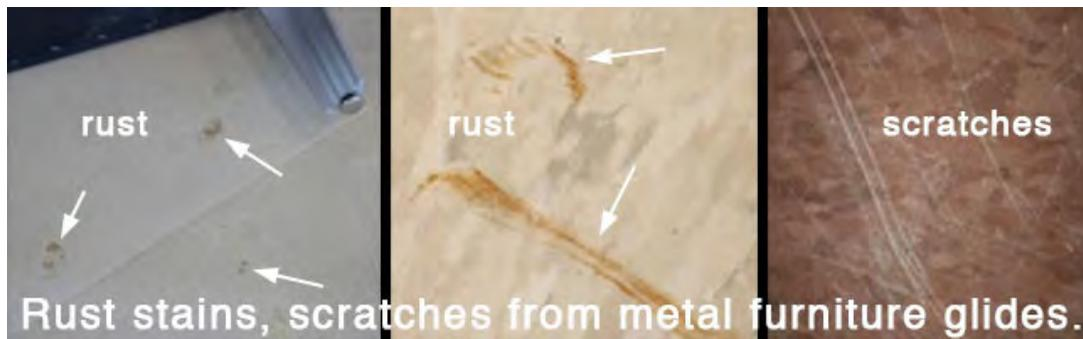
Plastic glides are hard and fragile resulting in broken remnants that contribute to severe flooring damage. Dirt and debris press into the surface of plastic protectors that can be more damaging than coarse sandpaper when the chair is repeatedly moved across the floor's surface.
